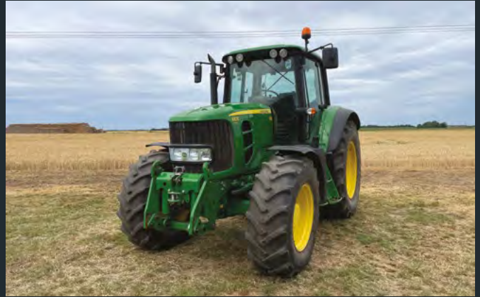
2011 John Deere 6830 Premium 4wd 40kph AutoQuad tractor with Degenhart front linkage, 3 manual spools, cab and front suspension on 420/85R28 front and 520/85R38 rear wheels and tyres. Hours: 3,142 - SOLD: £54,800
