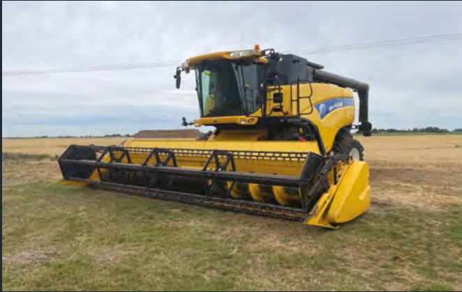
2010 New Holland CX8080 combine harvester with 25ft Varifeed header and trolley, straw chopper, 6 straw walkers, single side knife on 900/60R32 front and 540/65R30 rear wheels and tyres. Drum Hours: 1,710 - SOLD: £82,500
