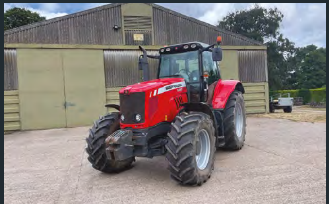
2011 Massey Ferguson 6485 Dyna-6 50kph 4wd tractor with 4 manual spools cab and front suspension and front wafer weights on 480/70R28 front and 580/70R38 rear wheels and tyres. Hours: 5,500 - SOLD: £35,000
